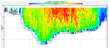
River discharge was determined from flow speed crosssection measurements collected using a towed ADCP
